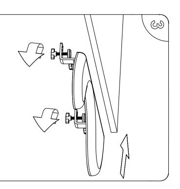
Install in the direction of the arrow and tighten the two hand screws
