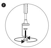
2. Hold the light pole as shown and tighten the side pin.
