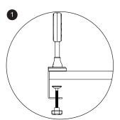
1. Place the clamp in place as shown and tighten the pin.
