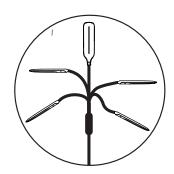
Hose can be bent according to the actual lighting needs, but not excessive distortion, excessive distortion will cause the hose deformation, restore Complex to less than the original, affecting the service life.
